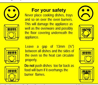
For the best results from the main oven we recommend that you use a baking tray which is 310mm (12") square. If you use a tray or tin which is larger than this, you may need to turn it around during cooking.
